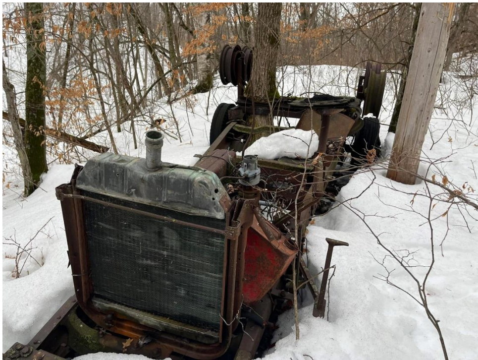
Relics of Engelwood Ski Area. Rope tows were powered by running a rope around the tire rim of an old car or truck that was set up on blocks.
